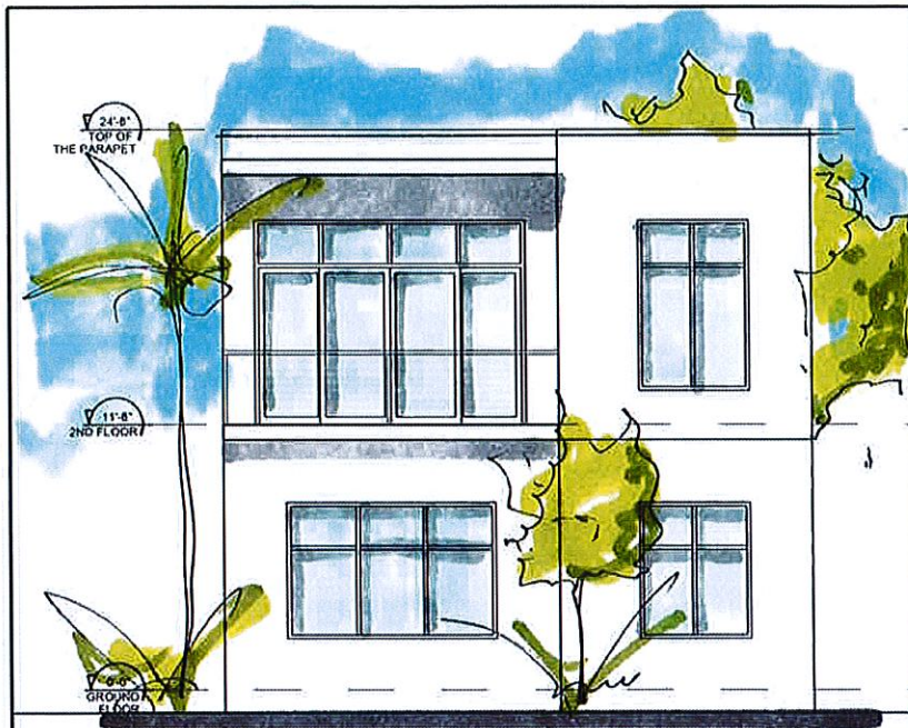
01 SOUTH ELEVATION - HOUSE TYPE C A-504 SCALE 1/4" = 1'-0"
